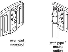
Fasten the DU to the bracket and verify that the signal strength (number of bars) is the same as observed in step 4.
