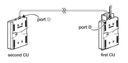
Connect power to the second CU and find a location for the unit (as shown in step 7) that displays the strongest level of coverage.
