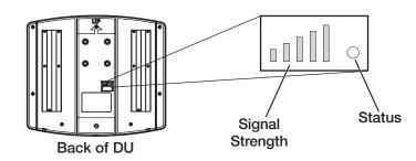
The DU should be mounted facing in the direction where the LED indicator shows the greatest numbers of bars and the Status LED is blue (no faults)
